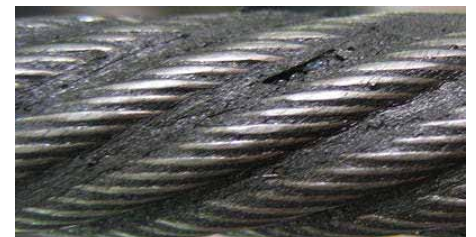
Left Lay - Counter Clockwise Rotation
